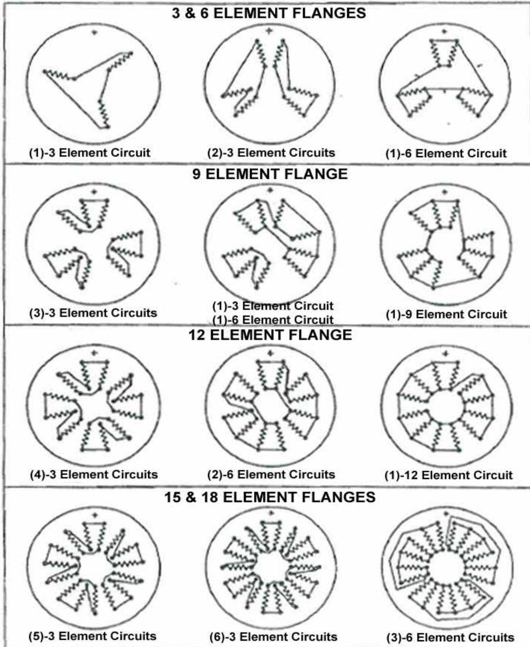
**FIGURE 4-3. Boiler Element Bussing Details**
