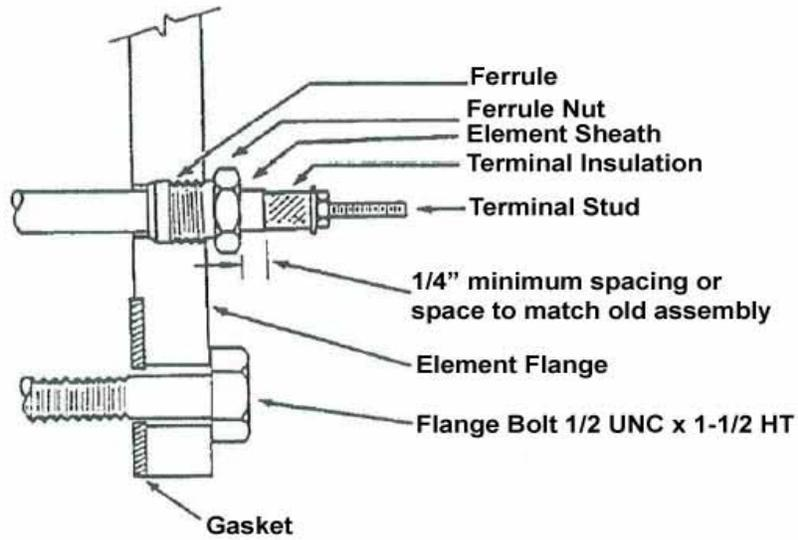
Ferrule is attached to ferrule nut until installation.
