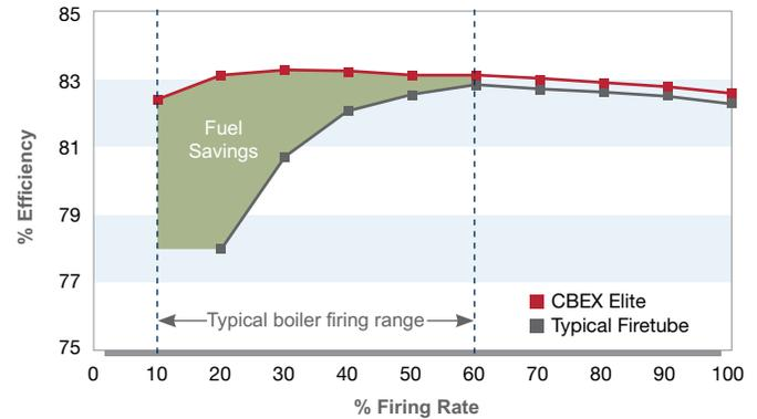
Recognizing this, in 1990, Cleaver-Brooks engineers made 10:1 turndown standard in its classic line of firetube boilers, featuring the industry's benchmark integral burner. With 10:1 turndown, a boiler can "turn down" to 10% of capacity without cycling, preventing needless energy losses.
