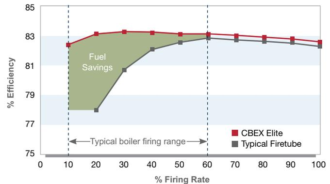
Efficiency curves based on natural gas firing at 125 psig steam at 30 ppm NOx. Efficiencies do not reflect secondary heat recovery options.
